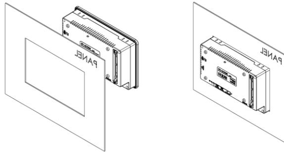
2. Insert the panel mount brackets into the bracket mounting holes as shown in the image below, pulling the bracket to lock it into place.
