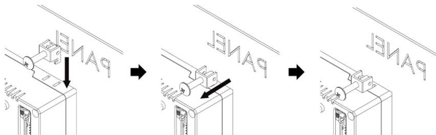
3. Tighten the bracket mounting bolts to secure the display to the panel. **The recommended torque is 0.4 Nm.**
